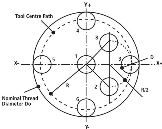
**1/2" x 14NPT internal thread in austenitic stainless steel using HX16 B 145 14NPT RS21**
